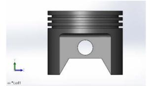
Fig. 3 Side view of the piston modeled
