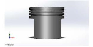
Fig. 4 Front view of the piston modeled
