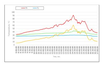
Fig. 8 Temperature dependence of hot-side of interior wall  $(T_h)$ , temperatures the water inlet  $(T_c)$ , Atmospheric temperature ( $T_a$ ), temperature difference ( $T_h - T_c$ ).
