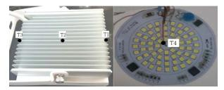
Fig. 3 Temperature measurement point.
