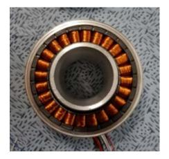
Fig. 9 Hollowed shafted BLDC motor
