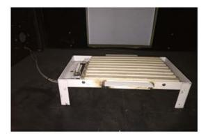
Fig. 2 Schematic diagram of the experimental apparatus. The right photo is the electrical heater placed into the chamber, which enables to maintain the indoor-outdoor temperature difference. This figure was copied from Ref. [6].
