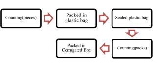
Fig. 5 Paper cup packing process
