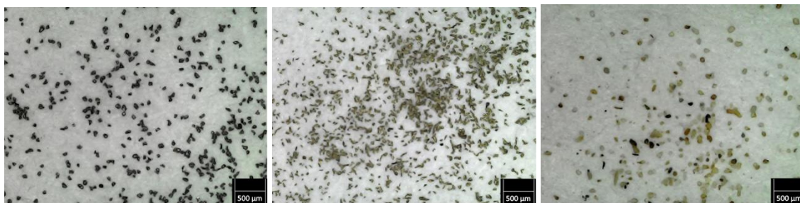
Figure 5 Typical images of solid (a) Ferrous particles, (b) Brass particles, (c) SiO 2 particles particles used in this study.
