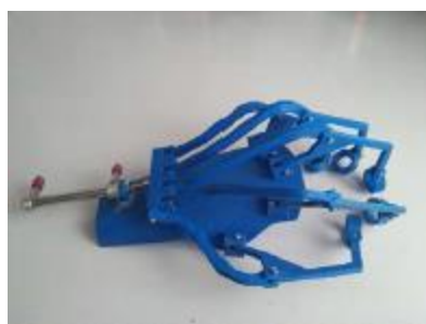
Figure 1 Serial linkage attached to distal hand exoskeleton
