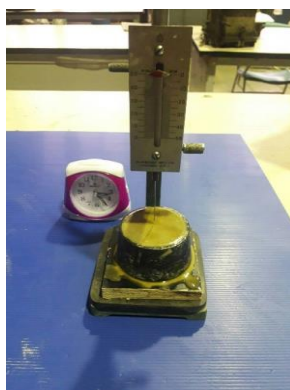
(b) Penetration resistance test
