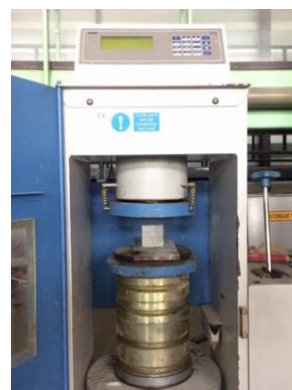
(c) Uniaxial compressive test
