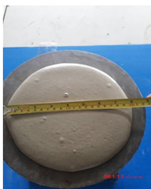
(a) Standard flow test
