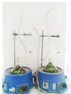
Figure 3 water distillation apparatus
