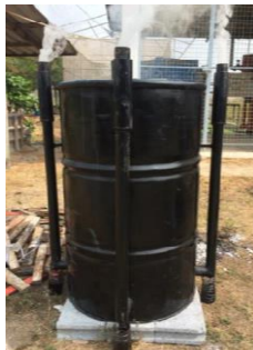
Figure 5 charcoal kiln
