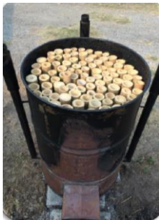
Figure 5 charcoal kiln
