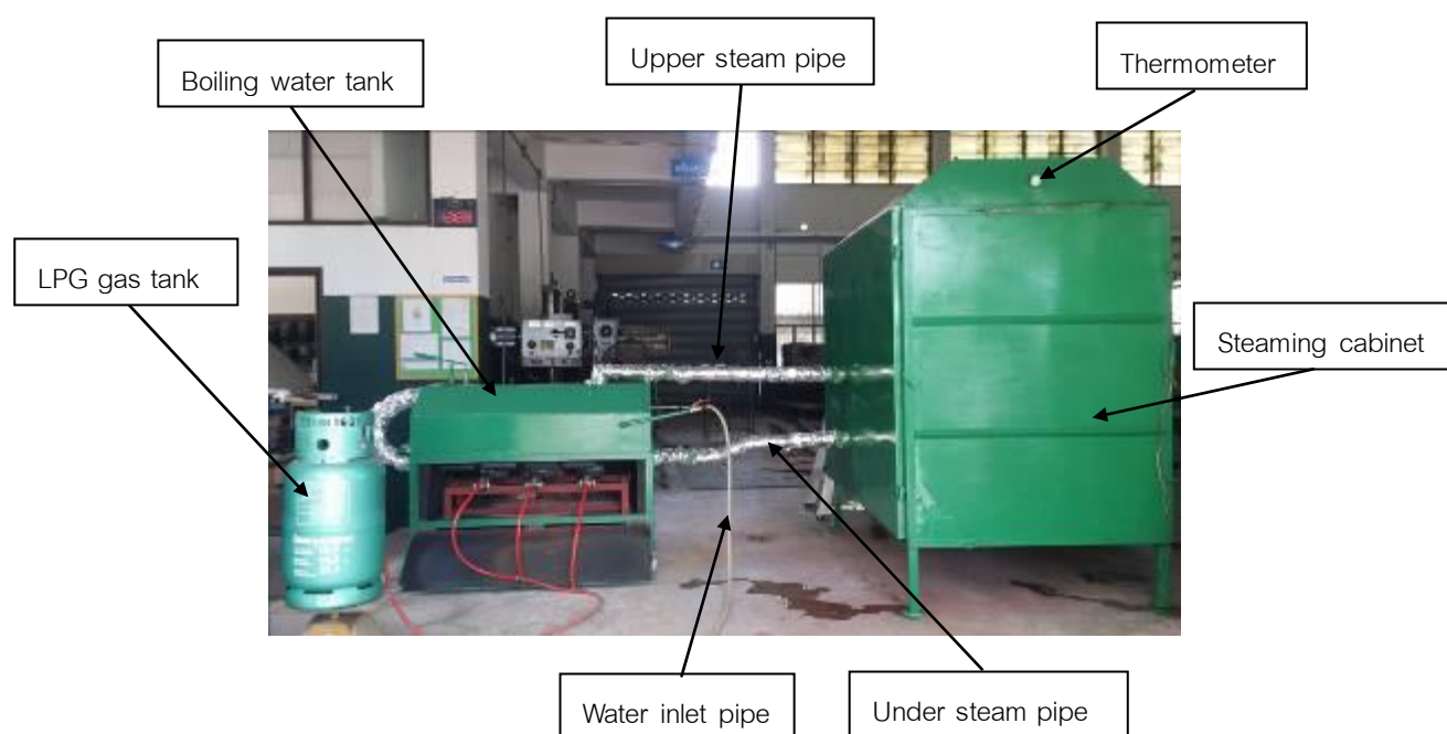
Figure 1 Dual powered mushroom compost steamer
